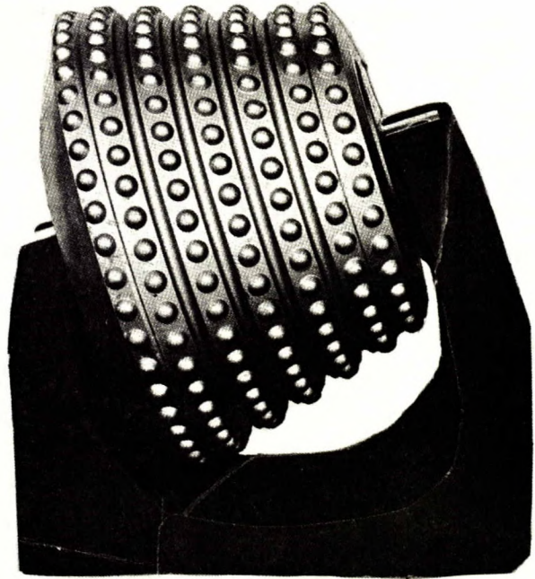
Rotating cutters with tungsten carbide buttons
