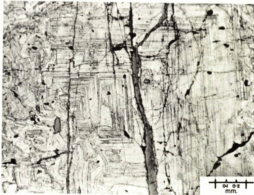
Figure 4. Photomicrograph showing complex zoning in magnetite, revealed by etching with concentrated HCl.
