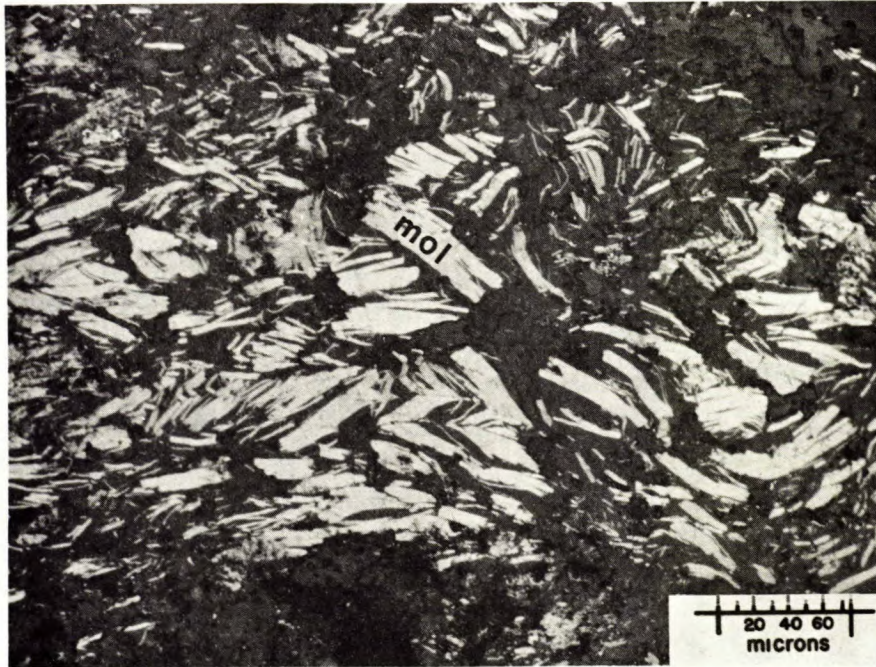
Figure 5. - Photomicrograph showing bundles of plate-like molybdenite (mol) grains in a predominantly quartz matrix.
