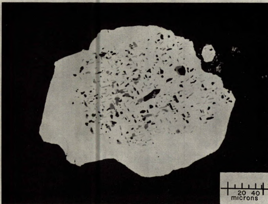
Figure 7. - Photomicrograph showing "ice-cake" texture between corroded pyrite (py) grains in a chalcopyrite (cp) matrix. Black areas represent pits.
