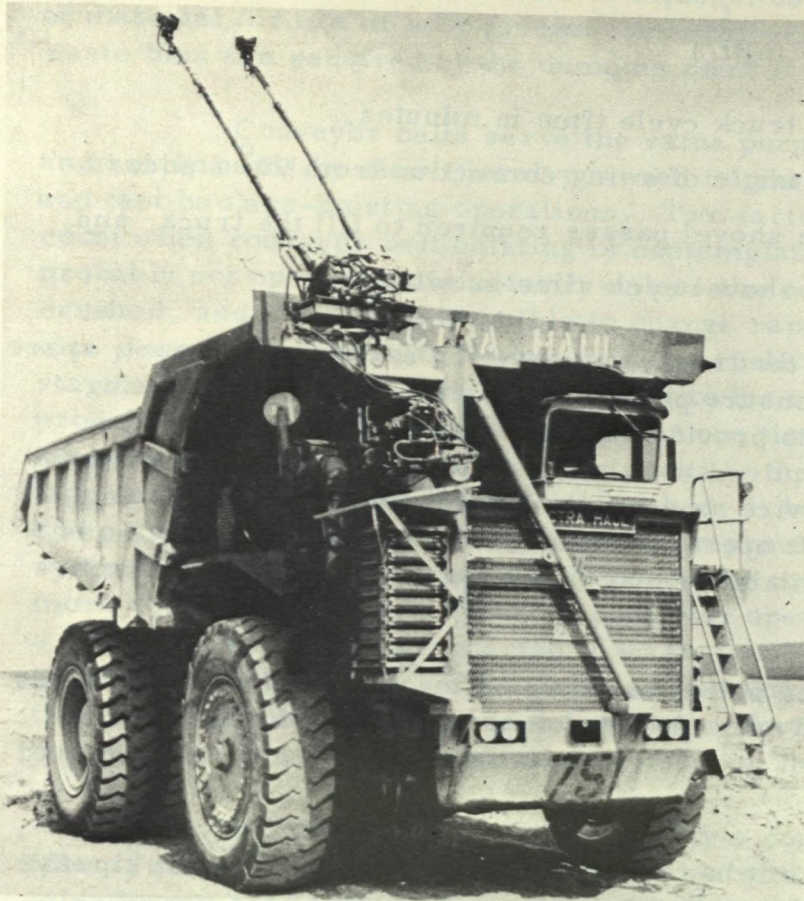
Figure 30. Haulage truck equipped with trolley poles. (Courtesy Quebec Cartier Mining Company)
