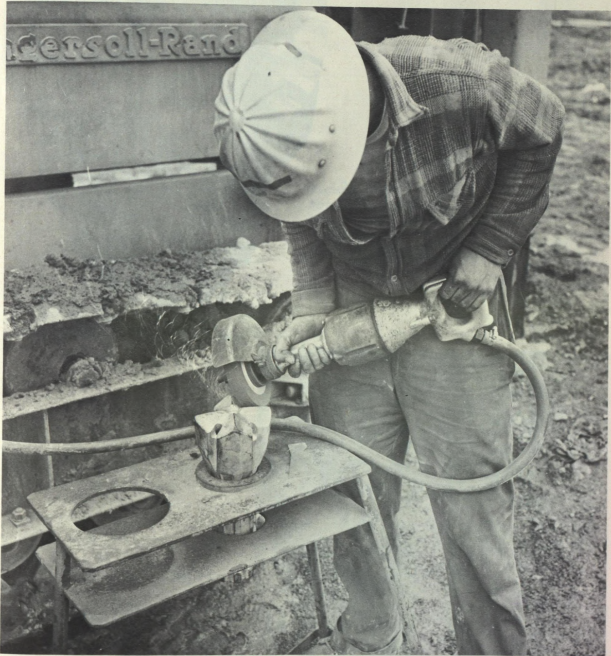
Figure 14. Hand sharpening a large-diameter percussion bit. (Courtesy Canadian Ingersoll Rand Company)
