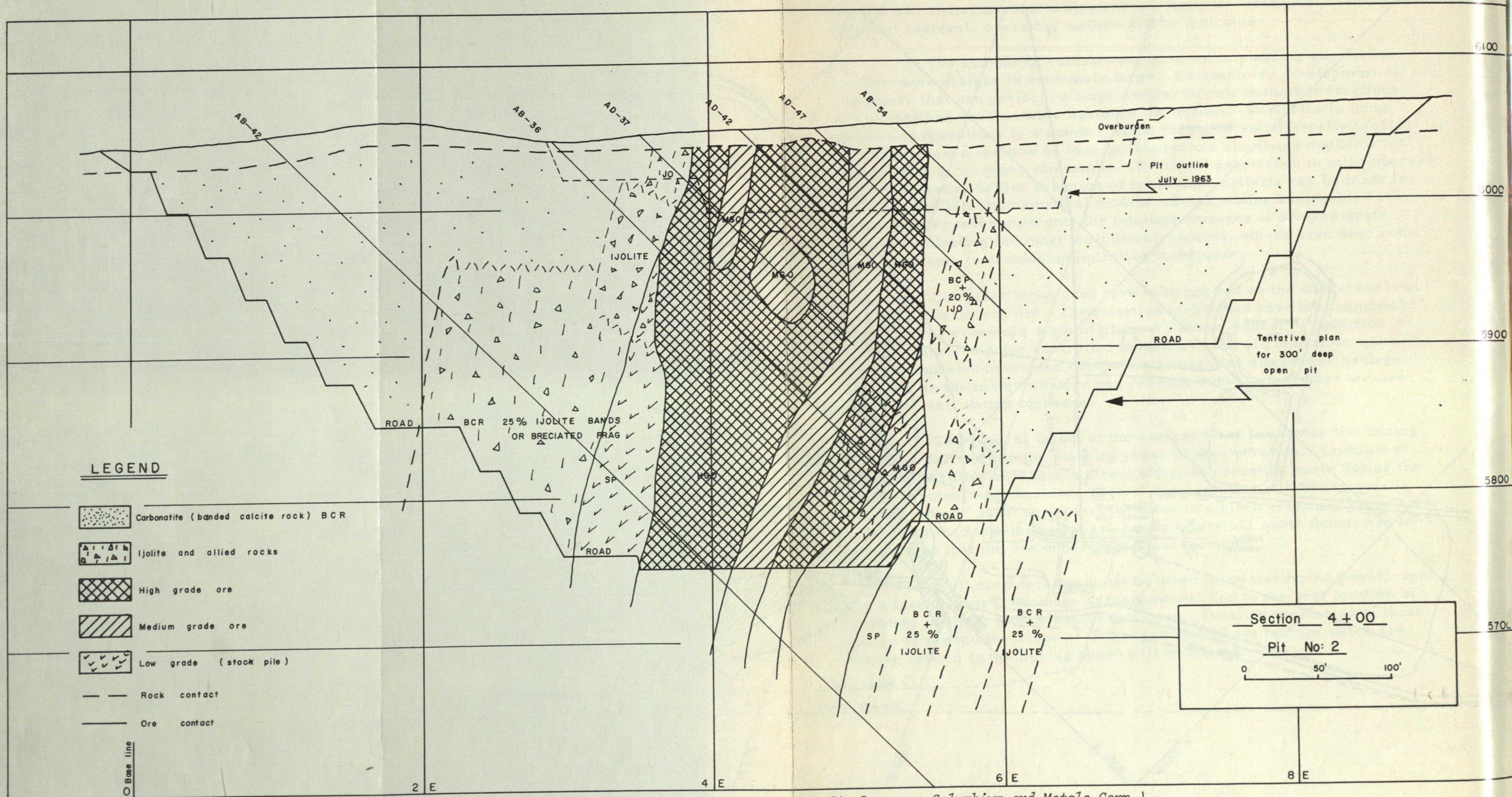
Figure 3. Section, idealized surface mine. (Courtesy St. Lawrence Columbian and Metals Corp.)
