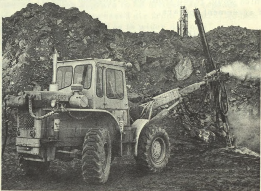
Figure 20. Specialized secondary drilling unit. (Courtesy Iron Ore Company of Canada)
