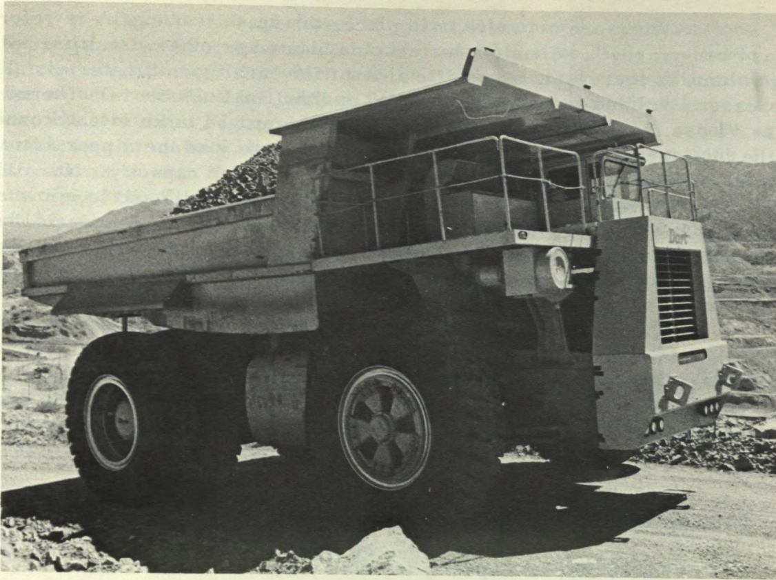
Figure 28. Two-axle rear-dump truck, 120-ton capacity. (Courtesy Sicard)
