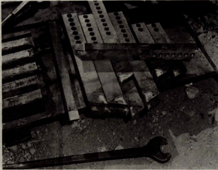
Figure 27. The carbide-tipped cutting knives, used as teeth in the cutterhead.
