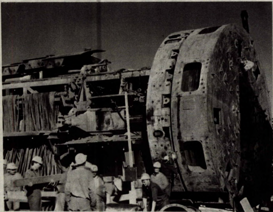
Figure 20. A side view of the cutterhead, with the wear ring and buckets removed.
