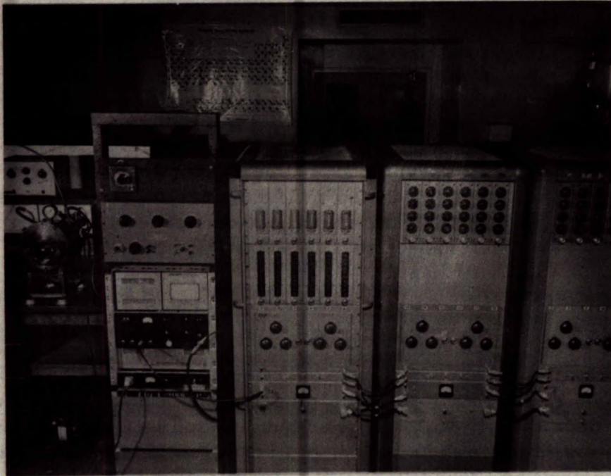
Figure 3. View of alpha-ray spectrometer. (Ionization chamber at extreme left, 18 channel kicksorter at right).
