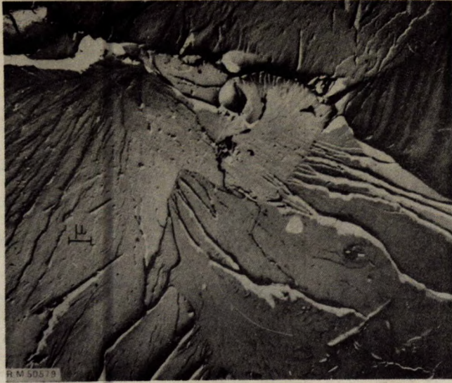
Figure 1 - River markings on cleavage surface in iron. (Ref. 2)
