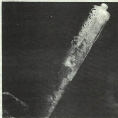
Fig. 4 High-temperature corrosion probe after the test with as-received crude oil
