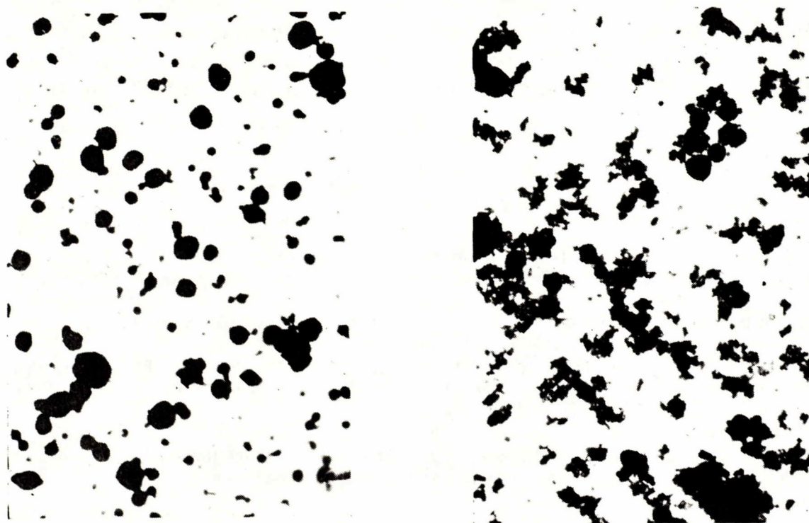
Fig. 4. Photomicrograph of soot particles. Magnification X160.
