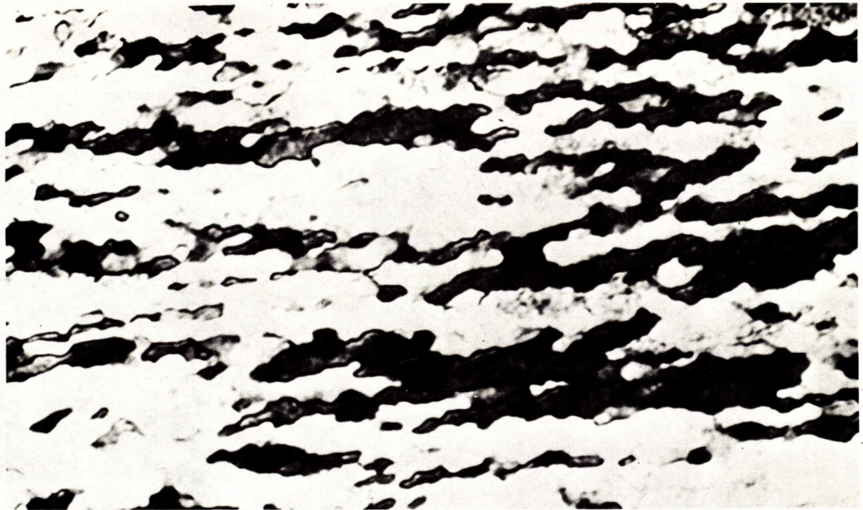
Figure 4. Microstructures observed under polarized light of aluminum hot-rolled at 0.55 Tm (150X) (a), (1000X) (b), and at 0.65 Tm (1000X) (c).
