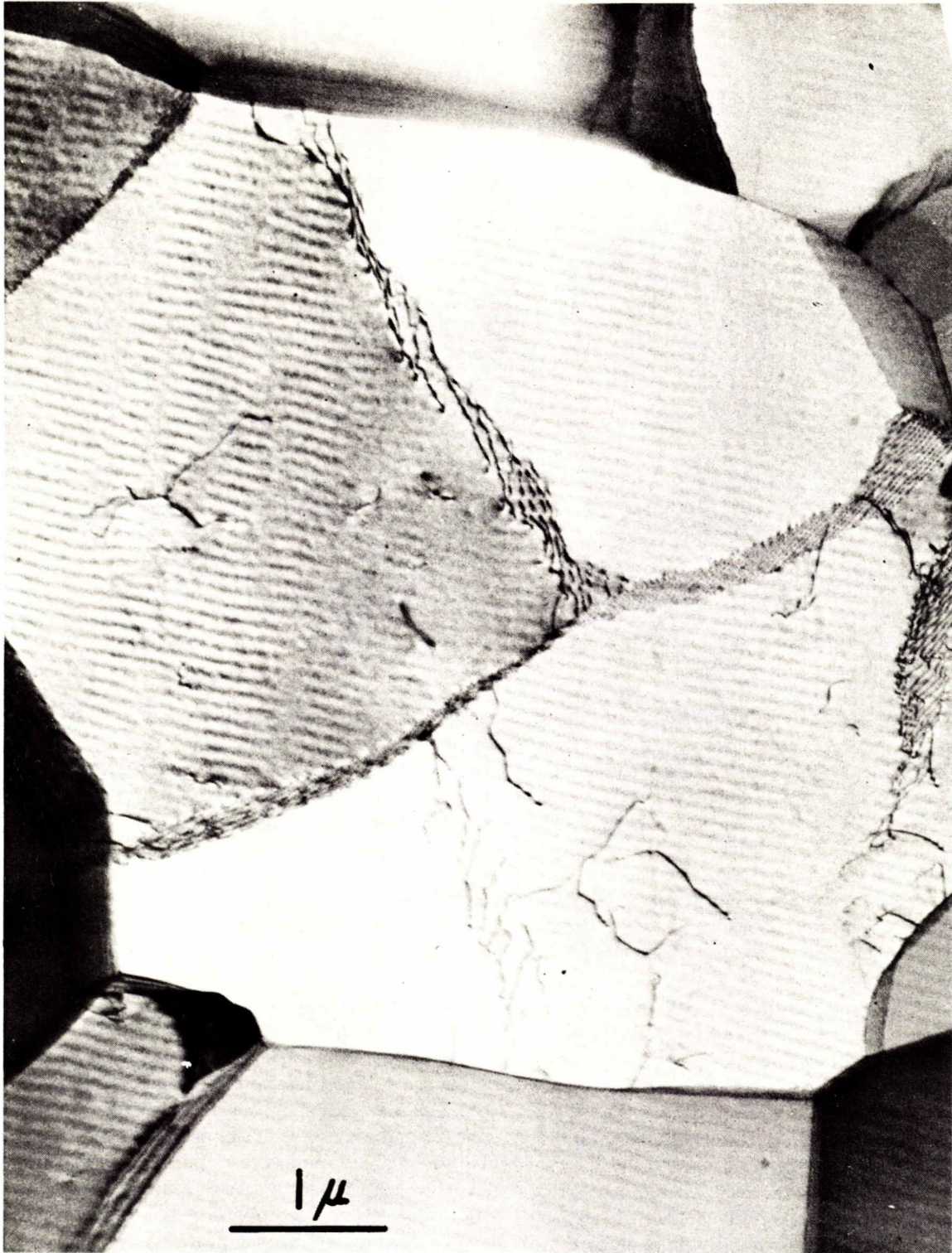
Figure 5. Electron micrographs of aluminum rolled at 0.55 Tm (a) and at 0.65 Tm (b).
