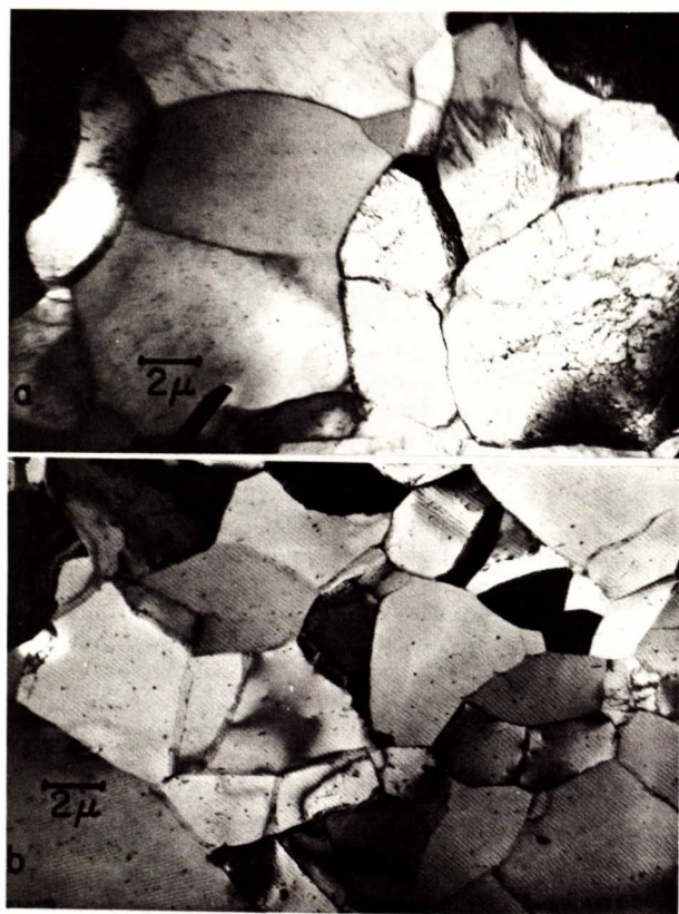
Figure 2. Subgrain diameter and perfection, in commercial purity aluminum extruded at 445°C, decrease with strain rate: (a) 0.5 sec -1 and (b) 5.5 sec -1 . Extrusion ratio 40:1.
