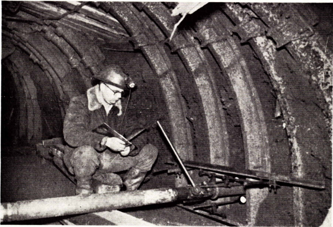
FIG. 3—Plate-load test on the wall of a drift.
