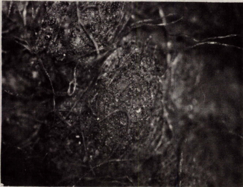
Figure 2b) Co-2, Cotton cloth after 50 cakes and thorough rinsing
