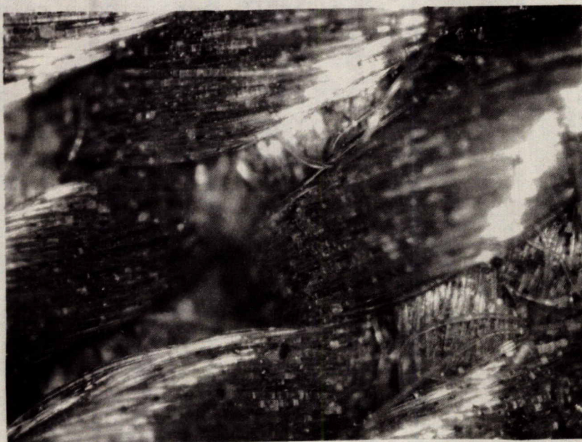
NY-2, Nylon cloth after 200 cakes. This cloth has identical flow characteristics after 200 cakes as it did after 50. The lack of loose fiber ends accounts for the lack of a permanently trapped layer.
