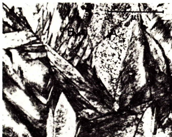
FIG. 2. Specimen oil-quenched from 1050°C—all micrographs from thin foils.
