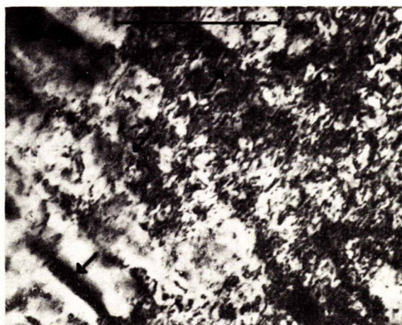
FIG. 3. Dislocations and cementite particles (arrowed) in quenched samples.
