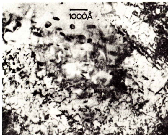
FIG. 13. Specimens tempered 120 hr at 600°C, showing dislocations clearing from centre of large plate-like grain.
