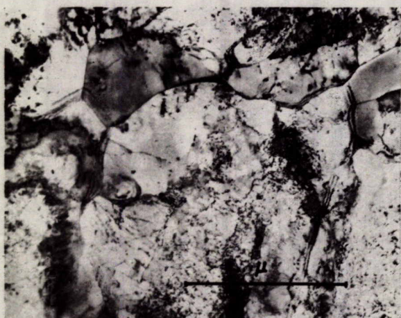
FIG. 16. Tempered 100 hr at 700°C, showing region from which dislocations have not cleared.
