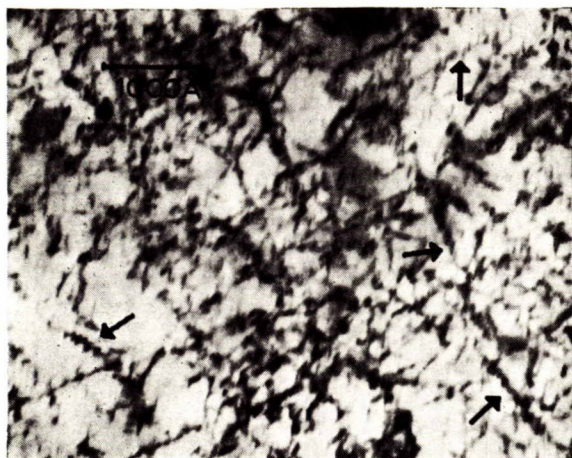
Fig. 17. Tempered 1 hr at 600°C. Arrows show particles aligned along dislocations.
