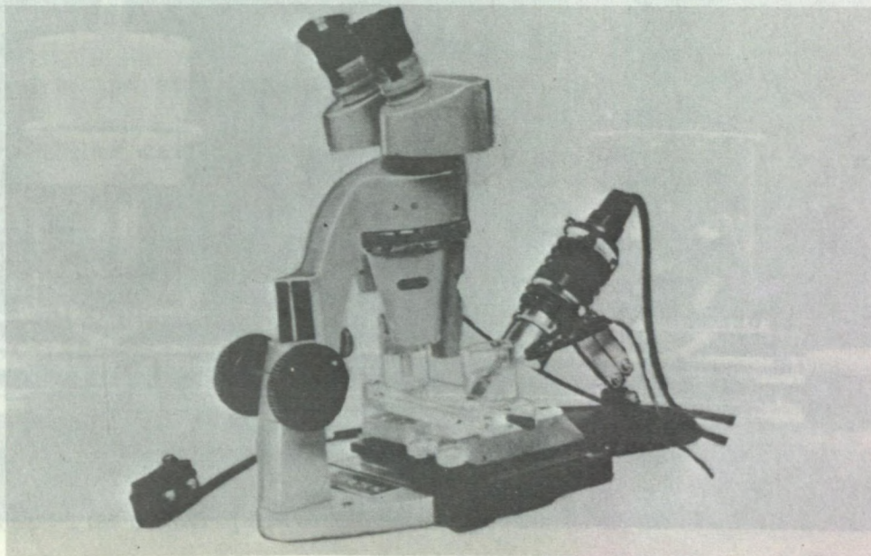
FIGURE 7. The Zeta-Meter Stereoscopic Microscope With Illuminator, Cell and Cell Holder, and Mechanical Stage.
