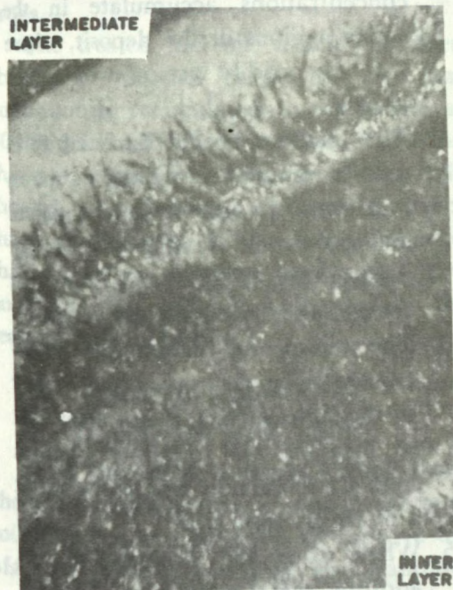
(c) Thin section of inner and intermediate upstream layers. Magnification X 15. Overall thickness 1.35 mm Inner layer thickness 0.07 mm
