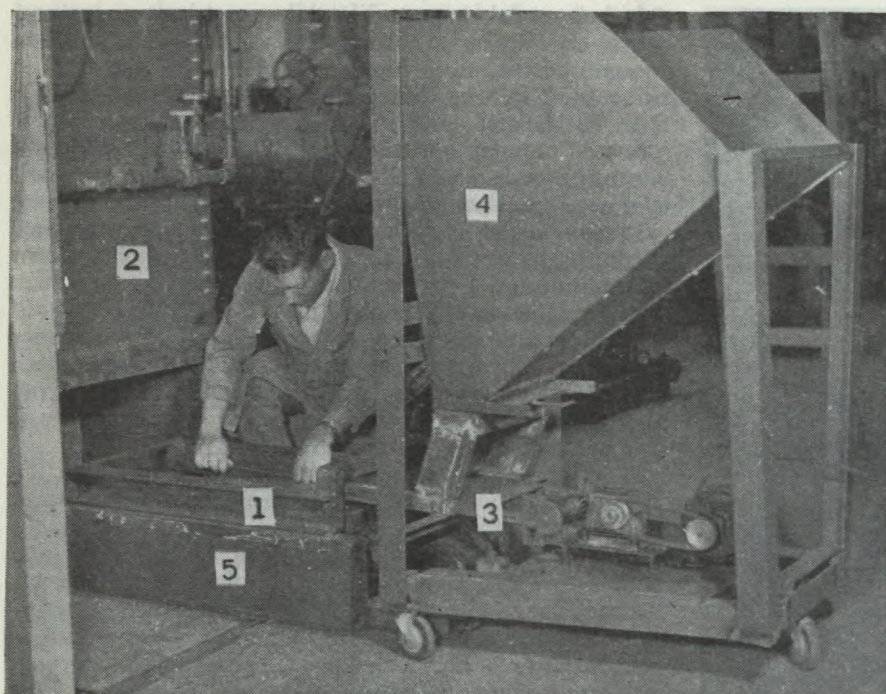
FIG. 4 (Left).—Assembly of grate, coal feeder and water-wall.
