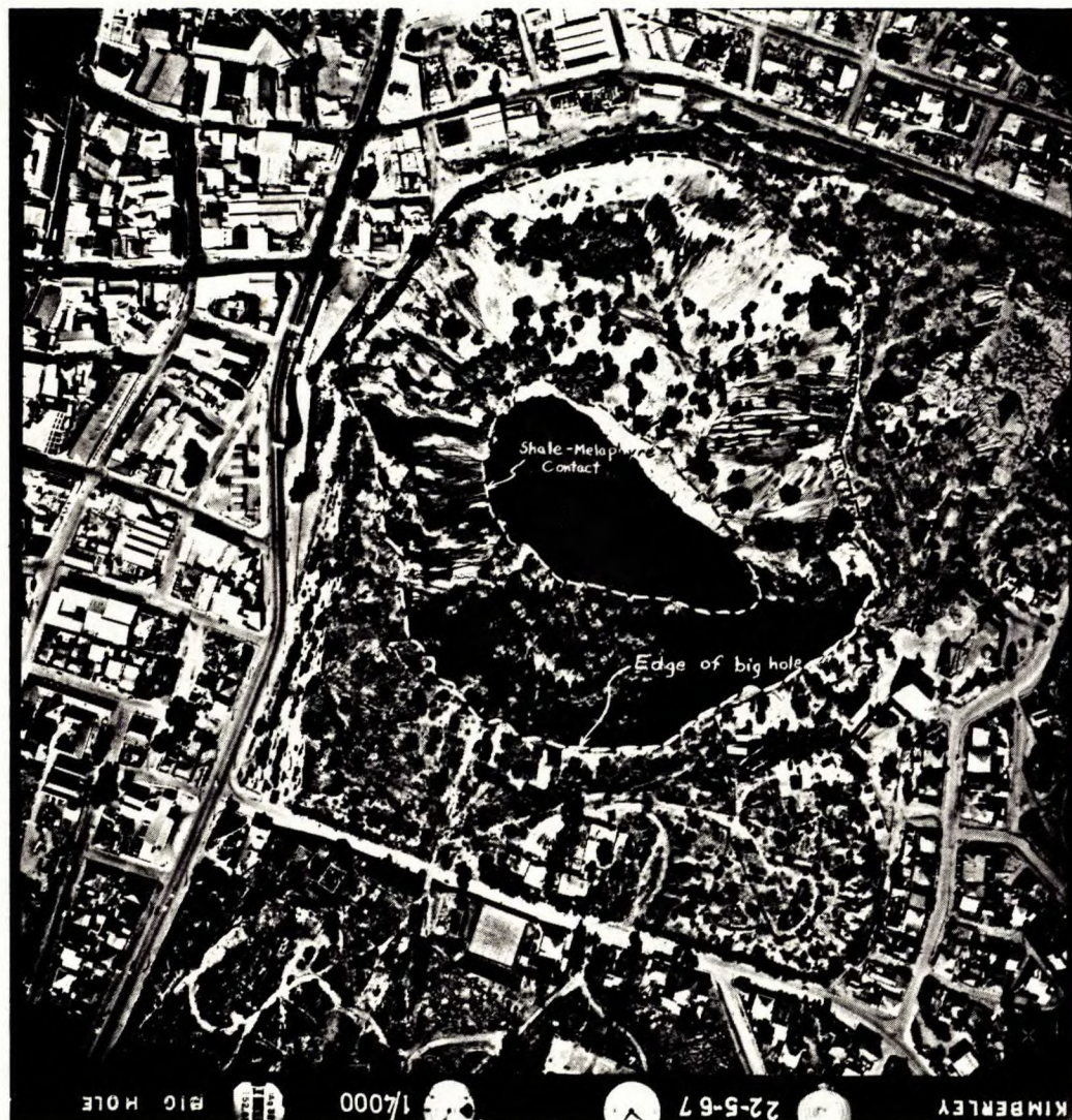
Photo 5. (i). Airphoto of the Kimberley Mine showing the plan outlines of the pipe at the shale-melaphyre contact and the edge of the "Big Hole".
