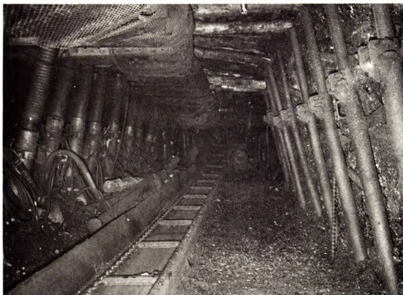
(f) Face C, after hand advance, before support advance
