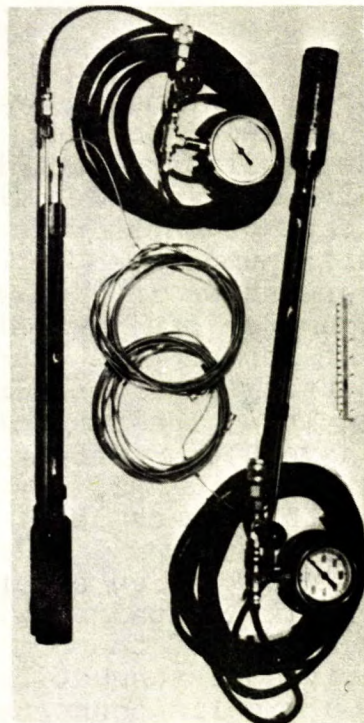
FIGURE 2 - Photograph of Sonic Transmitting and Receiving Units.
