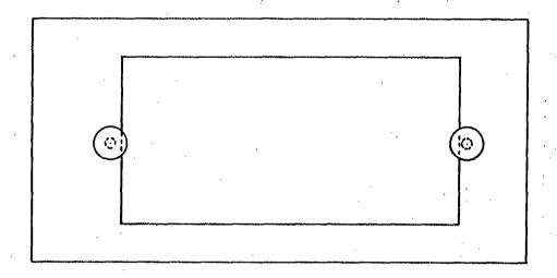
The plate holder used to immerse the plate in the etching solution is made of a plastic sheet 15 in.  $\times$  5 in.  $\times$  1/4 in. on which two Teflon retaining screws are mounted to hold the plates in position. This holder plate is clamped vertically in the etching tank.
