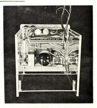
Provision can be made to have a printed front panel on which all controls are directly interconnected by printed connectors.
