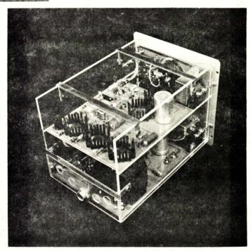
A rack was constructed to hold the standard printed circuit. It consists of two plastic plates, 7.3/4 in.  $\times 11.3/4$  in.  $\times 1/4$  in., with 1/8 in. grooves into which the modules slide. The two plates are retained at the proper distance by four strips of brass fixed in position by bolts. This rack can be housed in a Hammond # 1401F cabinet.
