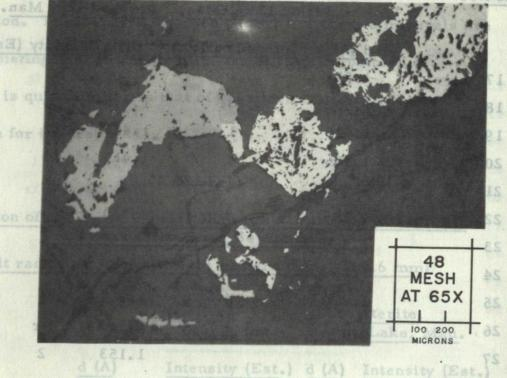
Figure 5. - Photomicrograph of polished section, showing grains of tapiolite (white) and microlite (light grey). Gangue minerals are dark grey and polishing pits are black.
