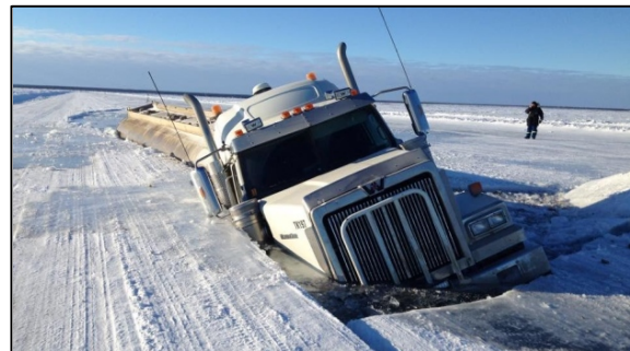
Fuel tanker breaks through lake ice on the winter road between communities of Deline and Tulita, Great Bear Lake, March 2016. Photo by GNWT Environment and Natural Resources.
