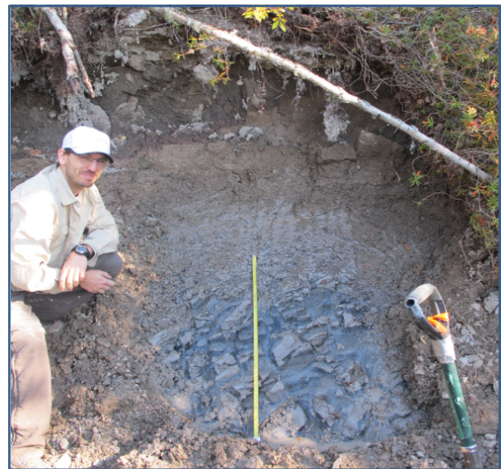
Ice exposed at the top of permafrost after surface materials have thawed. Philippe Normandeau, Northwest Territories Geological Survey. Photo by P. Morse.
