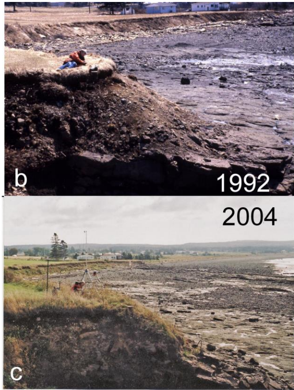
Figure 3. (a) Terrestrial and marine elevations can be related to a number of vertical datums including Ellipsoid, Geodetic and Chart. All elevations in this report are relative to Geodetic Datum, unless otherwise stated. (b, c) Elevations were derived from a tie-in survey to NS control monument 8270 (person and tripod) at the north end of the beach (Fig 2a).
