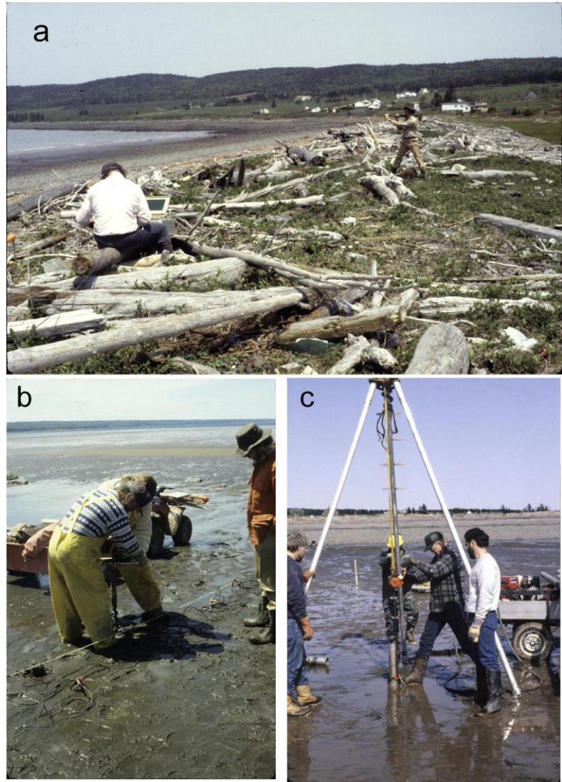
Figure 4. Sediment stratigraphy was obtained by using (a, b) seismic reflection surveys across the marsh, beach and tidal flat at line 4 which were ground truthed by (c) vibrocoring in the tidal flat and soil augering in the marsh (Fig.2b).
