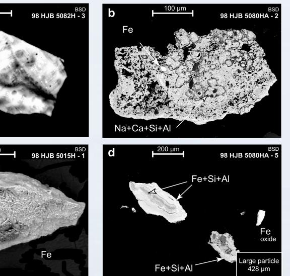
) smooth surfaced dusts with visible gas release bubbles or craters, botryoidal slag,corroded surface of a angular dust,
