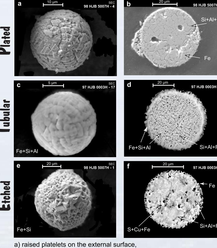
b) possible internal texture of agglomerated and partially melted dus c) dust surface is covered with short elongated tubes
