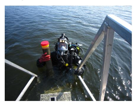
**Figure 4.** Hand-taken core from Lac Dasserat by a professional diver from Environment Canada during joint field work between Environment Canada and Natural Resources Canada; Photo: Environment Canada, Sept 2011
