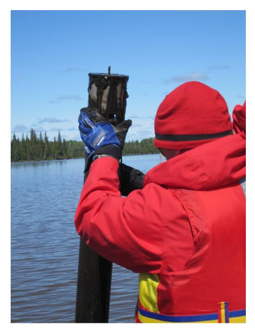
**Figure 12.** Sediment depth penetration was greater than the length of the core barrel, so that the sediments overflowed the top of the core barrel; the sediment-water interface was not preserved and the core discarded; Photo: Geological Survey of Canada, May 2012
