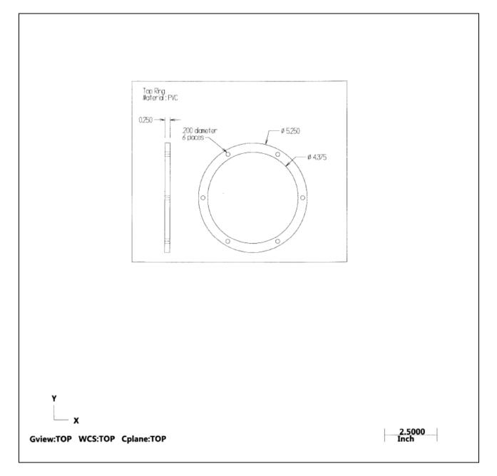
Figure B1. Technical drawing of the top ring of the depth control ring assembly (2 views)
