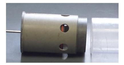
**Figure 6.** Auto valve on the head assembly of the Tech-Ops corer; Once the sediment seals the open end of the core tube, it creates a partial vacuum to prevent sediment from flowing out during ascent through the water column and retrieval. Photo: Geological Survey of Canada, May 2016
