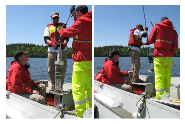
Figure 15. Routine operation of the modified Tech-Ops gravity corer; Photo: Geological Survey of Canada, May 2012
