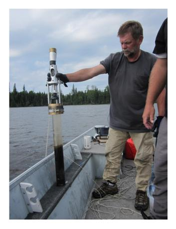
**Figure 2.** Deployment of the Glew corer in Lac Desvaux with insufficient core retrieval (< 30 cm); Photo: Geological Survey of Canada, July 2011
