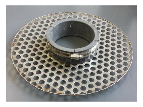
**Figure 9.** Photo of the custom-built stainless steel depth control ring, which attaches to the core barrel; Photo: Geological Survey of Canada, May 2016
