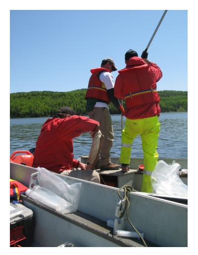
**Figure 8.** Attaching extension rod sections to the modified Tech-Ops gravity corer during its descent through the water column in Lac Dasserat; Photo: Geological Survey of Canada, May 2012
