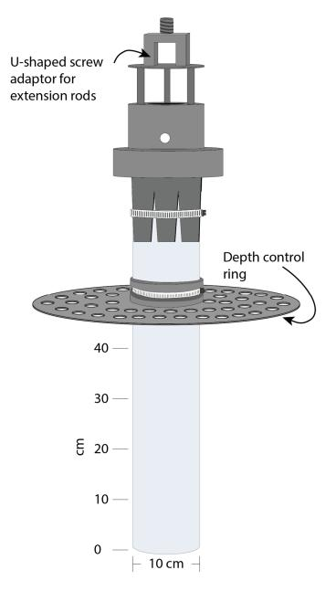
**Figure 10.** Tech-Ops gravity corer modifications – U-shaped adaptor for extension rods and depth control ring
