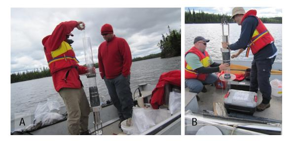
**Figure 13.** (A) Adjustable position of depth control ring; (B) Assembly of the modified corer; Photo: Geological Survey of Canada, May 2012
