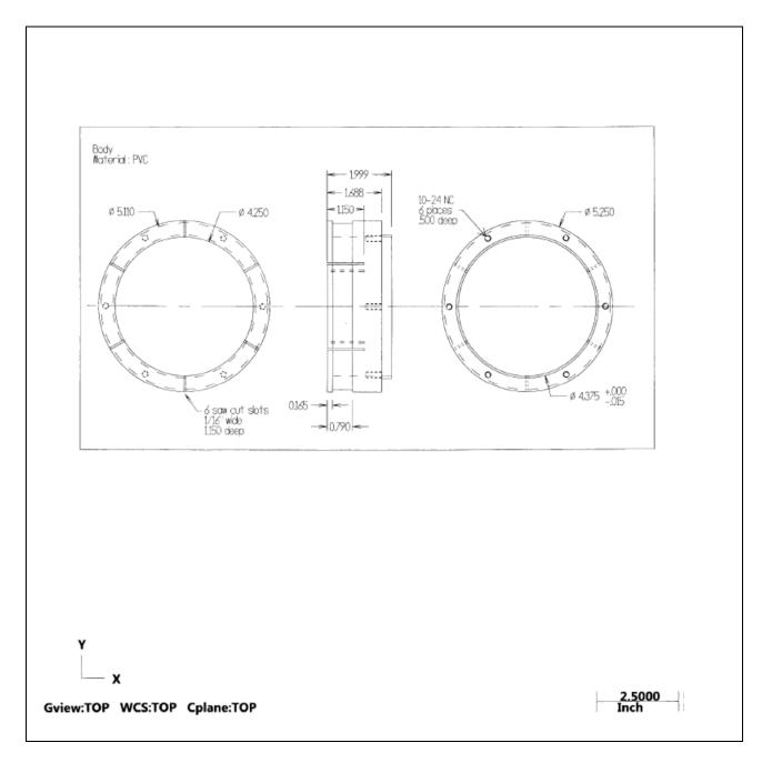
**Figure B3.** Technical drawing of the body collar which is the bottom attachment in the depth control ring assembly (3 views)
