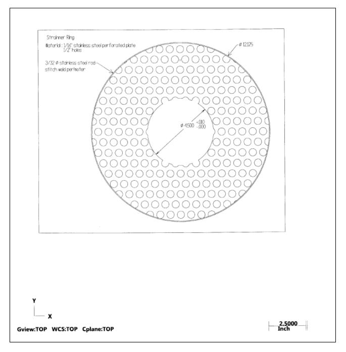
**Figure B2.** Technical drawing of the perforated depth control ring, sandwiched between the top ring (Figure B1) and the body collar (Figure B3)
