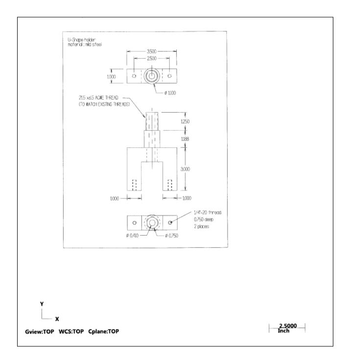
**Figure A1.** Technical drawing of the U-shaped steel screw adaptor for connection of threaded drive rods to the top of the Tech-Ops gravity corer (3 views)
