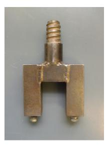
**Figure 7.** Photo of the custom-made steel U-shaped screw adaptor, which was mounted on the Tech-Ops corer head assembly to attach extension rods; Photo: Geological Survey of Canada, April 2016
