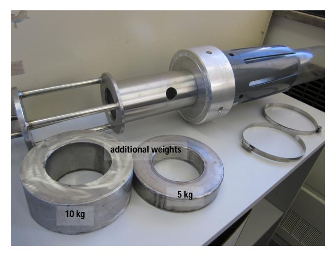
**Figure 5.** Unmodified Tech-Ops corer deployed in July 2011 without successful core retrieval in Lac Dasserat; Photo: Geological Survey of Canada, December 2010
