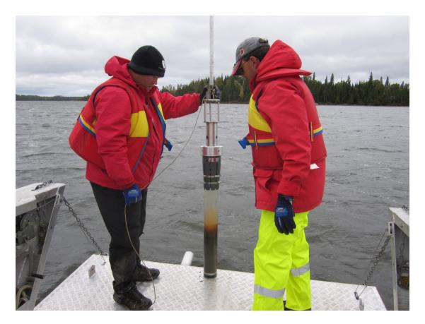
**Figure 11.** Successful coring with extension rods, although sediment depth was inadequate; Photo: Geological Survey of Canada, September 2011
