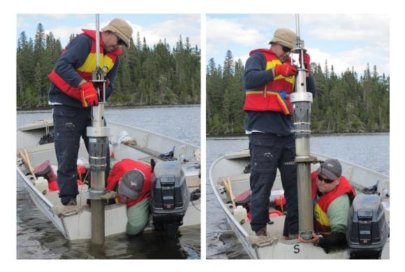
**Figure 16.** Insertion of the stopper into the bottom of the core tube upon retrieval with full modifications to the Tech-Ops corer; Photo: Geological Survey of Canada, May 2012
