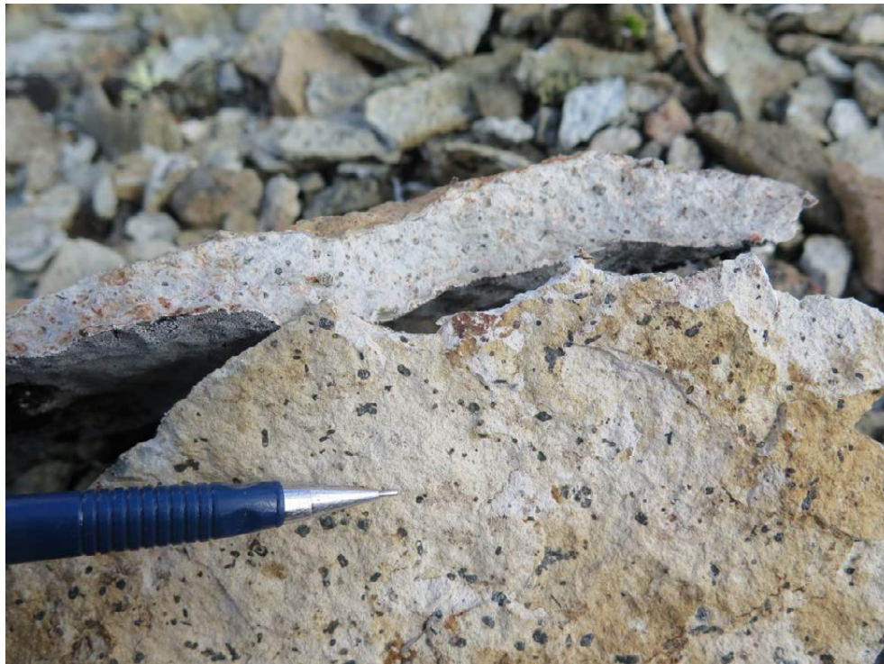
Figure 8: Quartz-feldspar porphyritic rhyolite of the Rhyolite Creek complex. Quartz phenocrysts in the photo are smoky to charcoal coloured. Pencil tip for scale.
