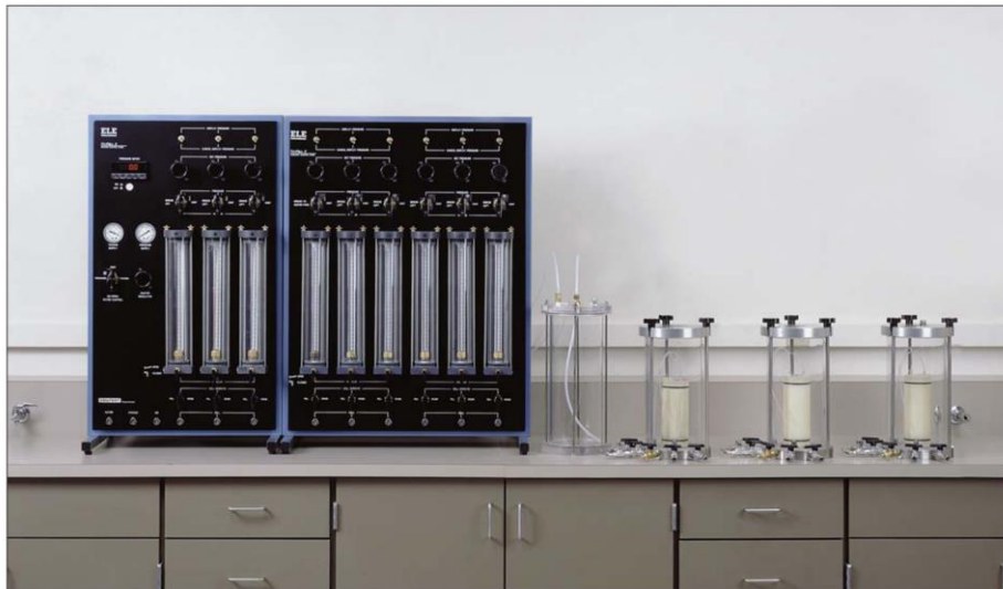
Figure 4. «Tri-Flex 2 Three Cell Permeability Test System » de ELE International
