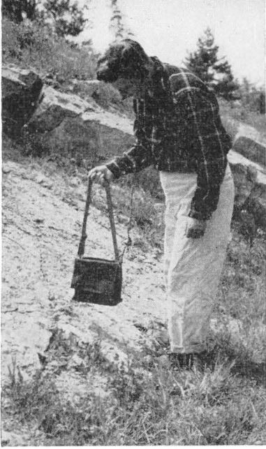
◀ A. Using counter with earphones to test outcrop.
