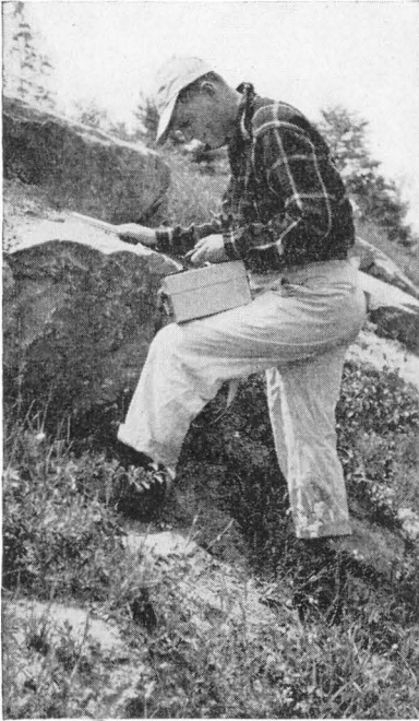
◀ B. Using counter with probe to test outcrop.
