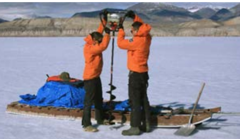
Parks Canada employees use an auger while measuring ice thickness on Lake Hazen in Quttinirpaaq National Park.
