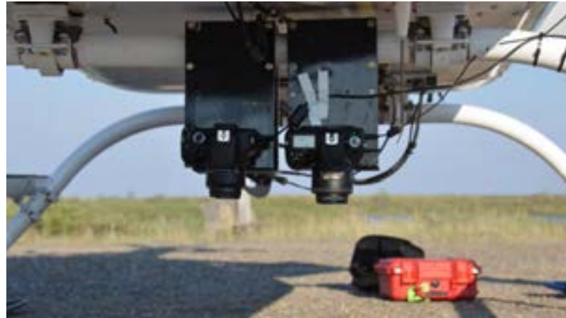
Cameras are mounted on a helicopter to take high-resolution air photos in the Mackenzie Delta region.
