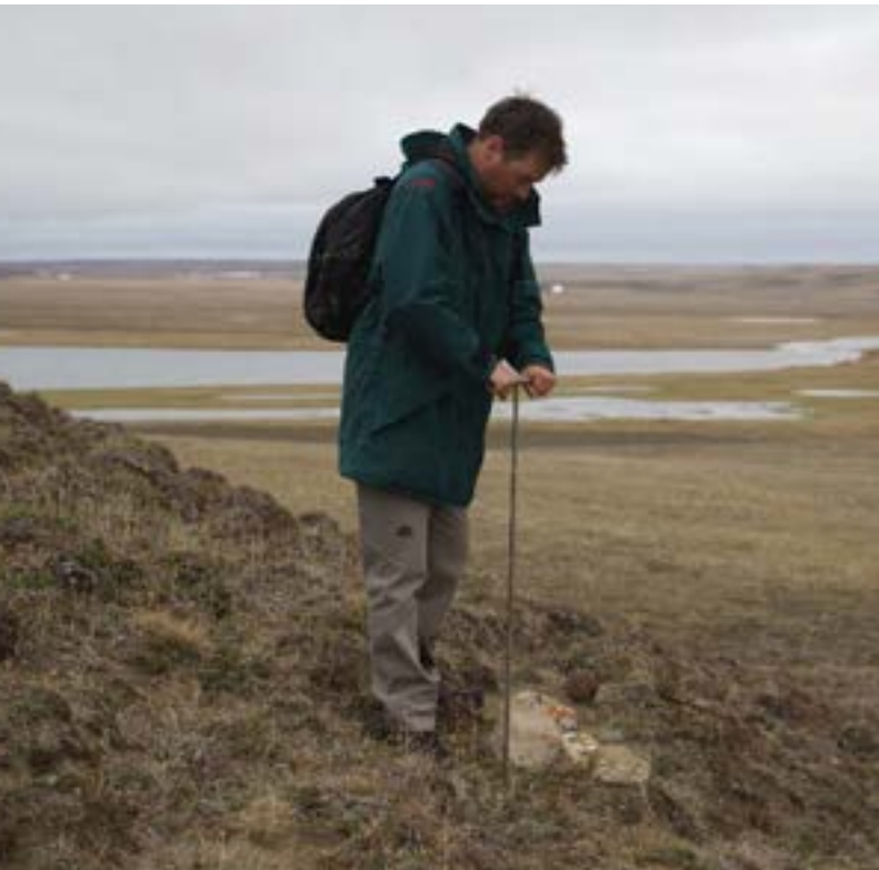
A Parks Canada employee uses a probe to measure active layer thickness in Aulavik National Park.
