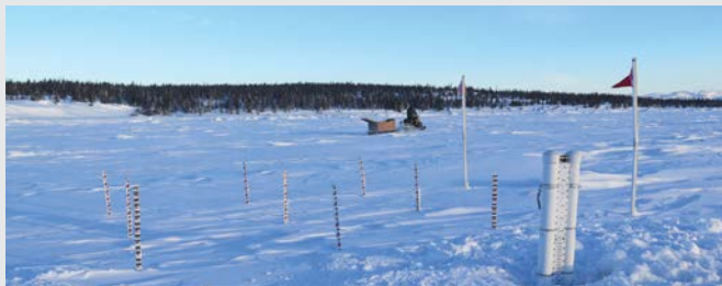
FIGURE 19: Community ice-monitoring station in Nain, NL, with a prototype SmartICE sensor frozen into the ice (right foreground). The sensor sends daily measurements of sea-ice thickness via satellite to the SmartICE data portal. Photo courtesy of R. Briggs.
