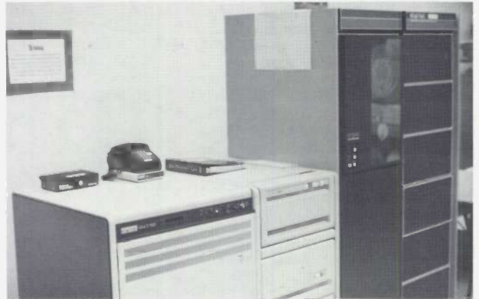
VAX 11/750 computer with disk drive, tape drive and expansion cabinet. Surveys and Mapping Branch, Manitoba
