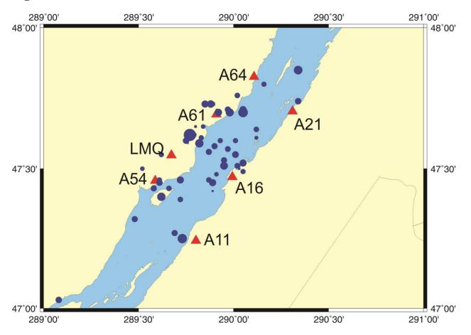
**Figure 1.** Map showing earthquakes (blue circles) used to develop the magnitude relations. Symbols size is scaled to magnitude (range -0.6 to 4.1). The red triangles show the locations of seismograph stations in the Charlevoix Seismic Zone.
