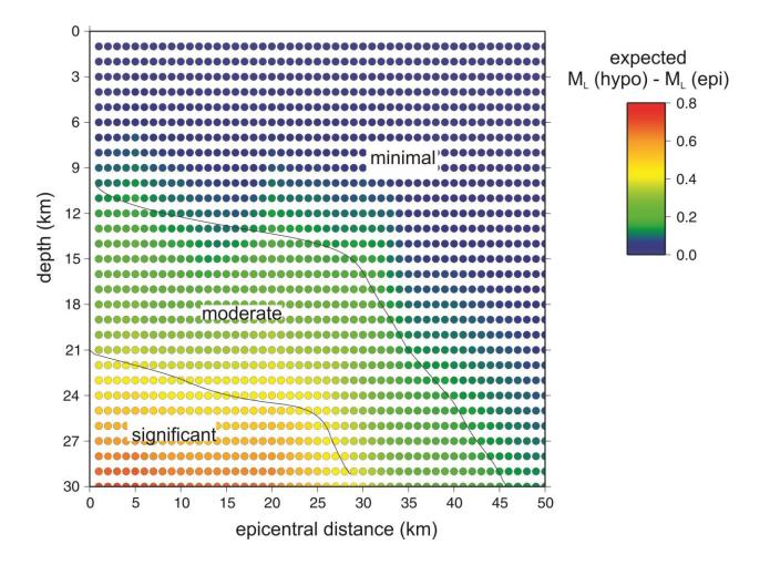
**Figure 3.** The difference in  $M_L$  magnitudes calculated for hypocentral and epicentral distances for a range of depths and distances. The labels showing ranges significant, moderate and minimal difference are qualitative only.
