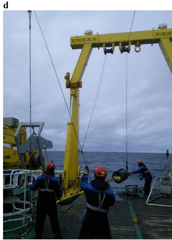
Figure 6.3 - Photos of heat probe. (a) and (b) a hook is newly attached just above the barrel tip for easy handling during winch operation. Size and direction of the hook is determined not to bother contact of thermistor with sediments when the probe is penetrated into sediments. The probe is deployed and recovered with cooperation of two winches to avoid damage of the thermistors from crush to ship. (c) before and (d) after hook attachment.
