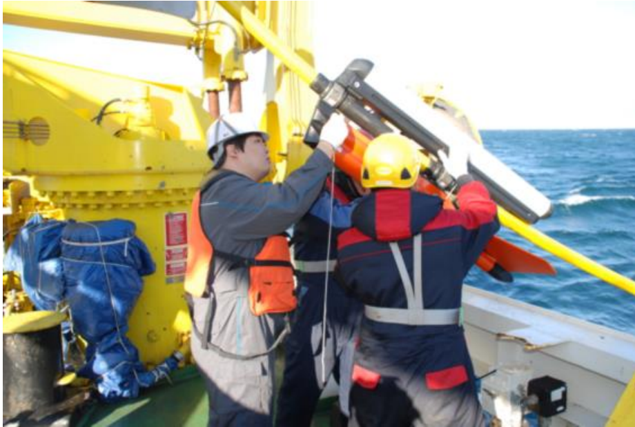
Figure 3.5 - Launching the streamer. The cable leveler (bird) is attached and tested on the streamer.
