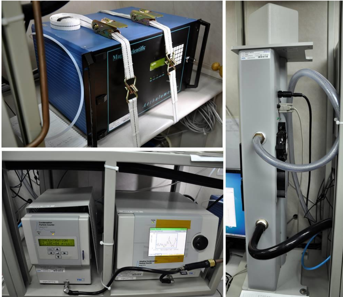
Figure 11.5 - Aerosol measuring instruments: (Up-left) Aethalometer, (Bottom-left) Condensation Particle Counters (CPC3772 and CPC3776), and (Right) Nephelometer.
