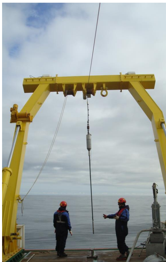
Figure 8.1 - SW-CPTu instrument on A-frame of RV Araon prior to deployment on cruise ARA05C.
