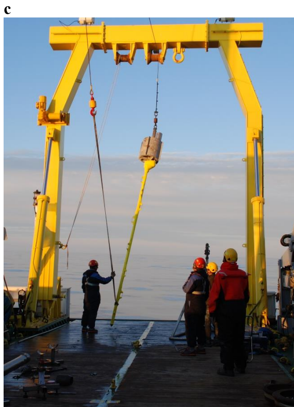
Figure 6.3 - Photos of heat probe. (a) and (b) a hook is newly attached just above the barrel tip for easy handling during winch operation. Size and direction of the hook is determined not to bother contact of thermistor with sediments when the probe is penetrated into sediments. The probe is deployed and recovered with cooperation of two winches to avoid damage of the thermistors from crush to ship. (c) before and (d) after hook attachment.
