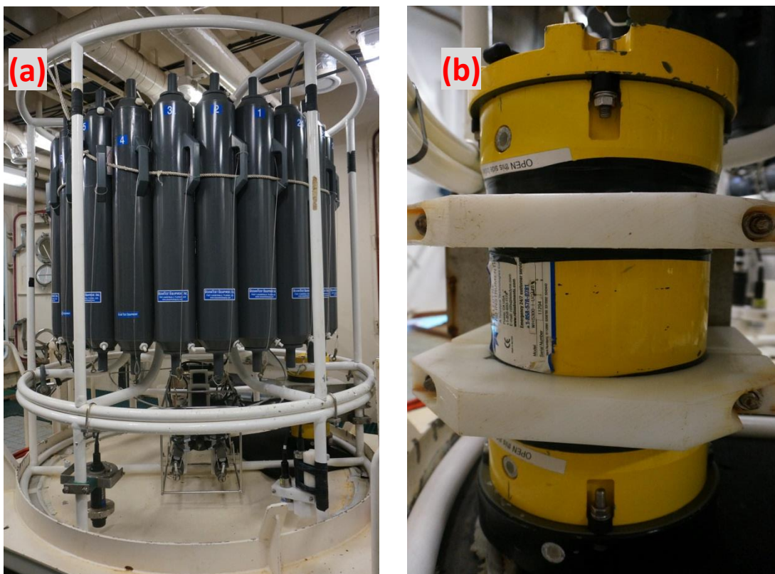
Figure 9.2 - Hydrographic observation equipment: (a) SBE911plus CTD profiler and rosette water sampler, (b) 300 kHz RDI lowered ADCP.
