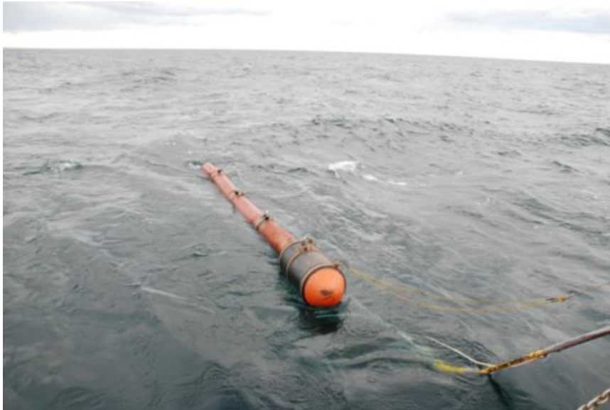
Figure 3.4 - Airgun array is launched on the sea. A float (red color tube) maintains the source depth at 6 m in the water.
