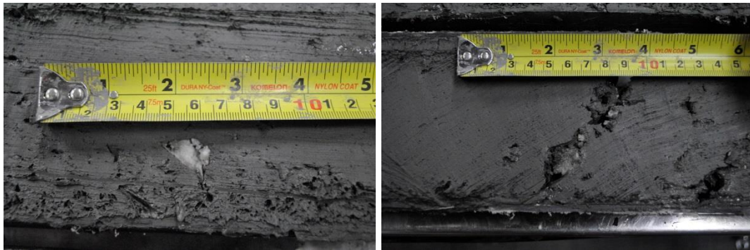
Figure 7.11 - Gas hydrates in core ARA05C 18GC01 from the 740 m water depth mud volcano.
