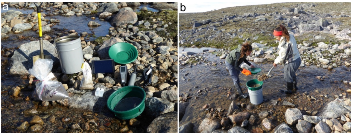
Figure 4. a) Samples collected and field equipment used at a typical bulk stream sediment and water site. b) Sieving sediments along an unnamed stream in the northwest quadrant of NTS 56A.
