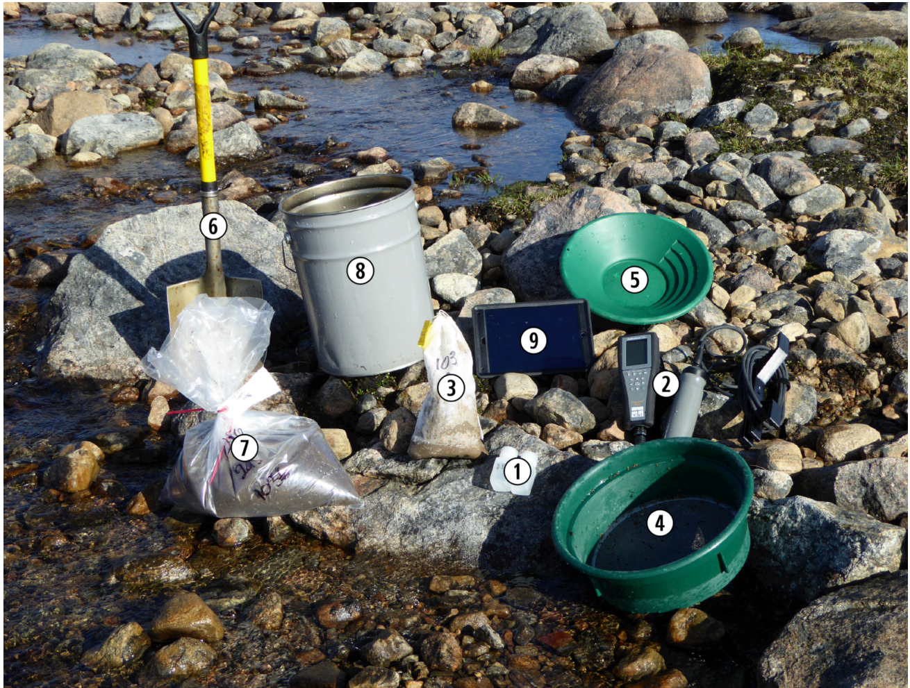
Figure 2: Field gear used and samples collected at a typical bulk stream sediment and water site.
