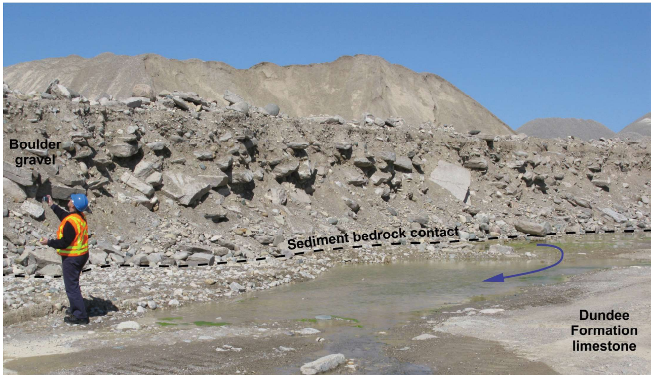
Figure 12.11 Groundwater flows from the interface or contact zone aquifer. This Interface aquifer consists of boulder gravel directly overlying Dundee Formation limestone. Meteoric water has percolated downward through the highly permeable gravel to the upper surface of the nearly impermeable limestone, and is flowing toward the viewer on the slightly inclined bedrock surface. Note that sand and silt was removed from above the boulder gravel.
