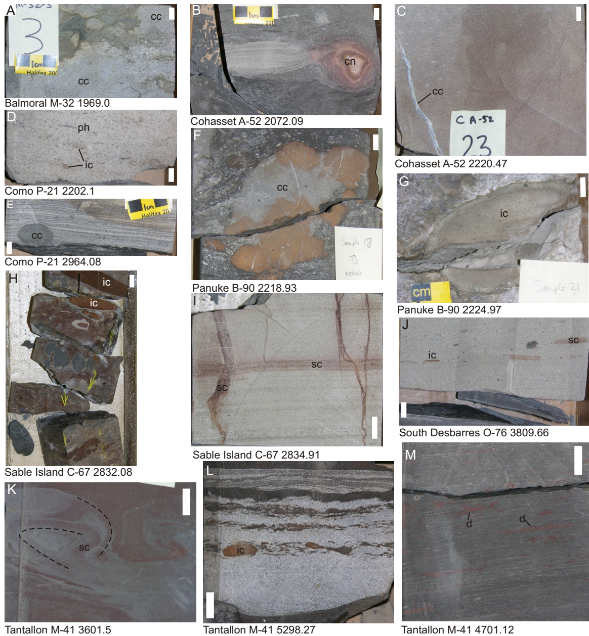
Figure 2: Core photos of representative samples from the studied wells. A: Balmoral M-32-1969.0: Greenish fine grained sandstone with carbonate patches; B: Cohasset A-52-2072.09: Concretion in shale; C: Cohasset A-52-2220.47: Fine grained sandstone with a calcite vein; D: Como P-21-2202.10: Coarse grained sandstone with one of several small sorted detrital siderite intraclasts scattered through the rock together with some phytoclasts; E: Como P-21-2964.08: Large carbonate cemented concretion in sandstone; F: Panuke B-90-2218.93: Carbonate concretion with a composite bioclast (visible in thin section); G: Panuke B90-2224.97: Carbonate intraclast; H: Sable Island C-67-2832.08: Carbonate intraclast (intraclast conglomerate); I: Sable Island C-67-2834.91: Fine grained sandstone
