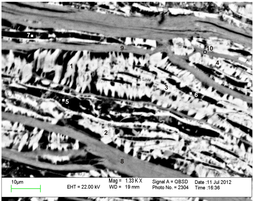
Figure 7A.22a. South Desbarres 0-76 3809.66m (SEM). Siderite (mostly type 5, but few of type 4) rhombohedrons formed between and perpendicular to the cleavage plane of the replaced framework mineral (probably muscovite). This figure is a higher magnification of figure 21.
