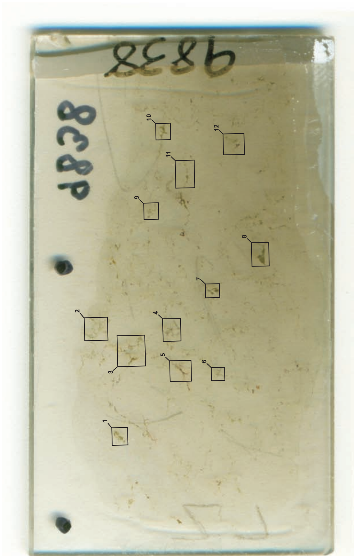
Figure 2-3A: Scanned polished thin section of sample 9838 with the locations of the studied fractures.
