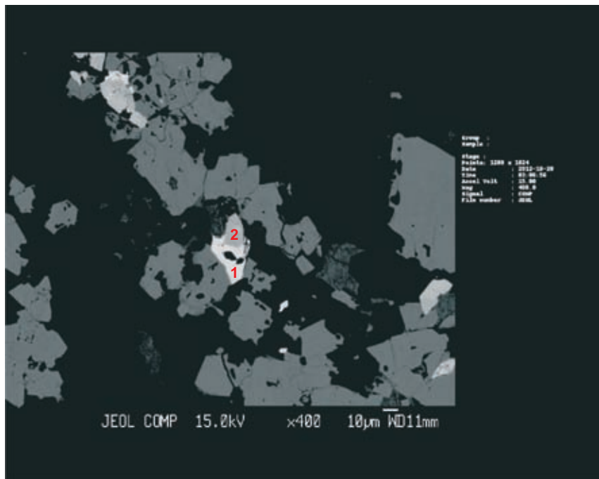
Figure 1-3.6b: West Moose River Pluton 9835 WDS analysis spots; precipitation of xenotime (analysis 1) postdates that of Fe-oxides (dark phase) and zircon (analysis 2). Xenotime contains over 15 wt.% HREE.
