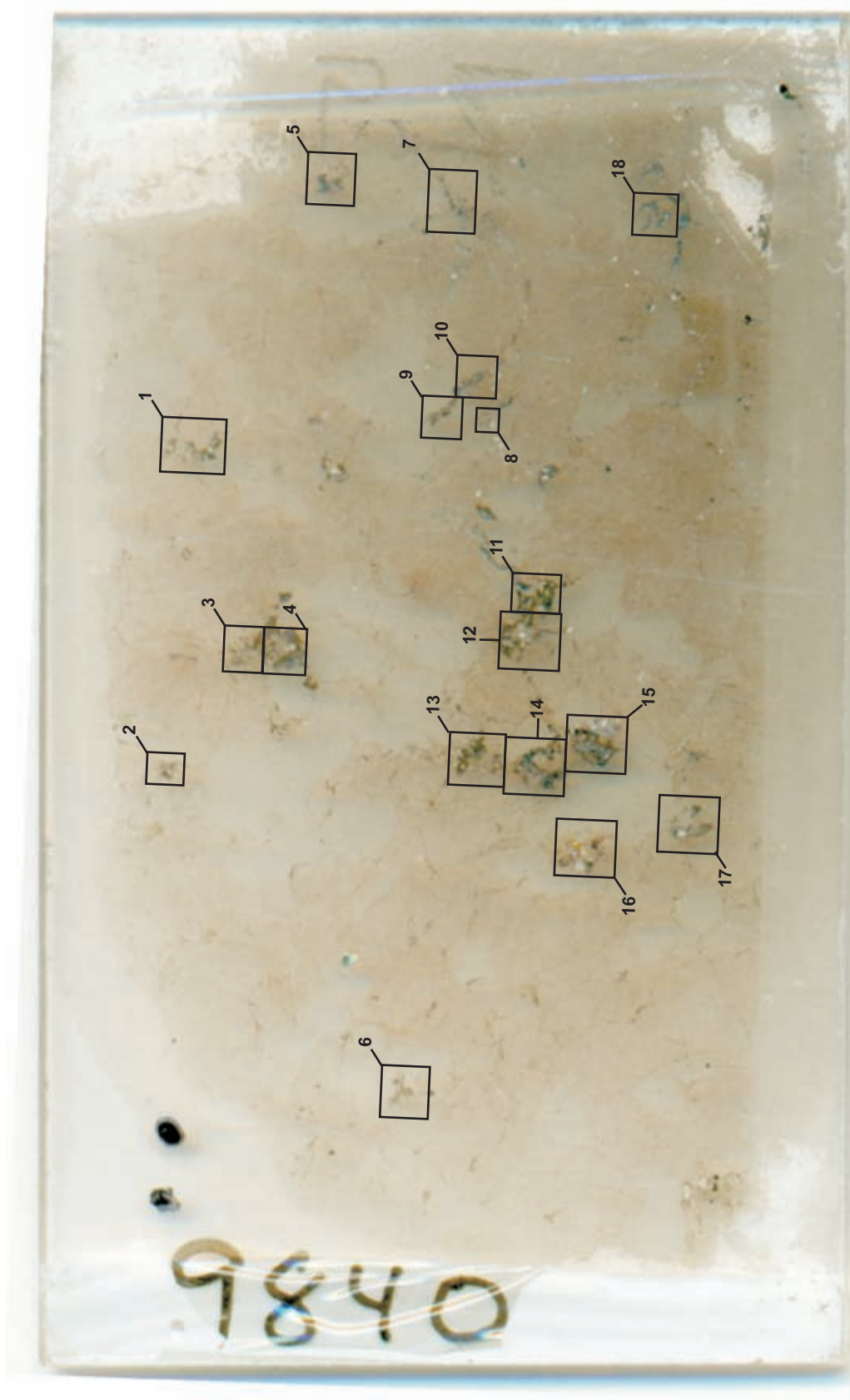
Figure 2-4A: Scanned polished thin section of sample 9840 with the locations of the studied fractures.
