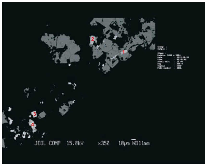
Figure 1-3.2b: West Moose River Pluton 9835 WDS analyses; hingganite (analysis 4) is associated with xenotime (analysis 3) in a fracture.
