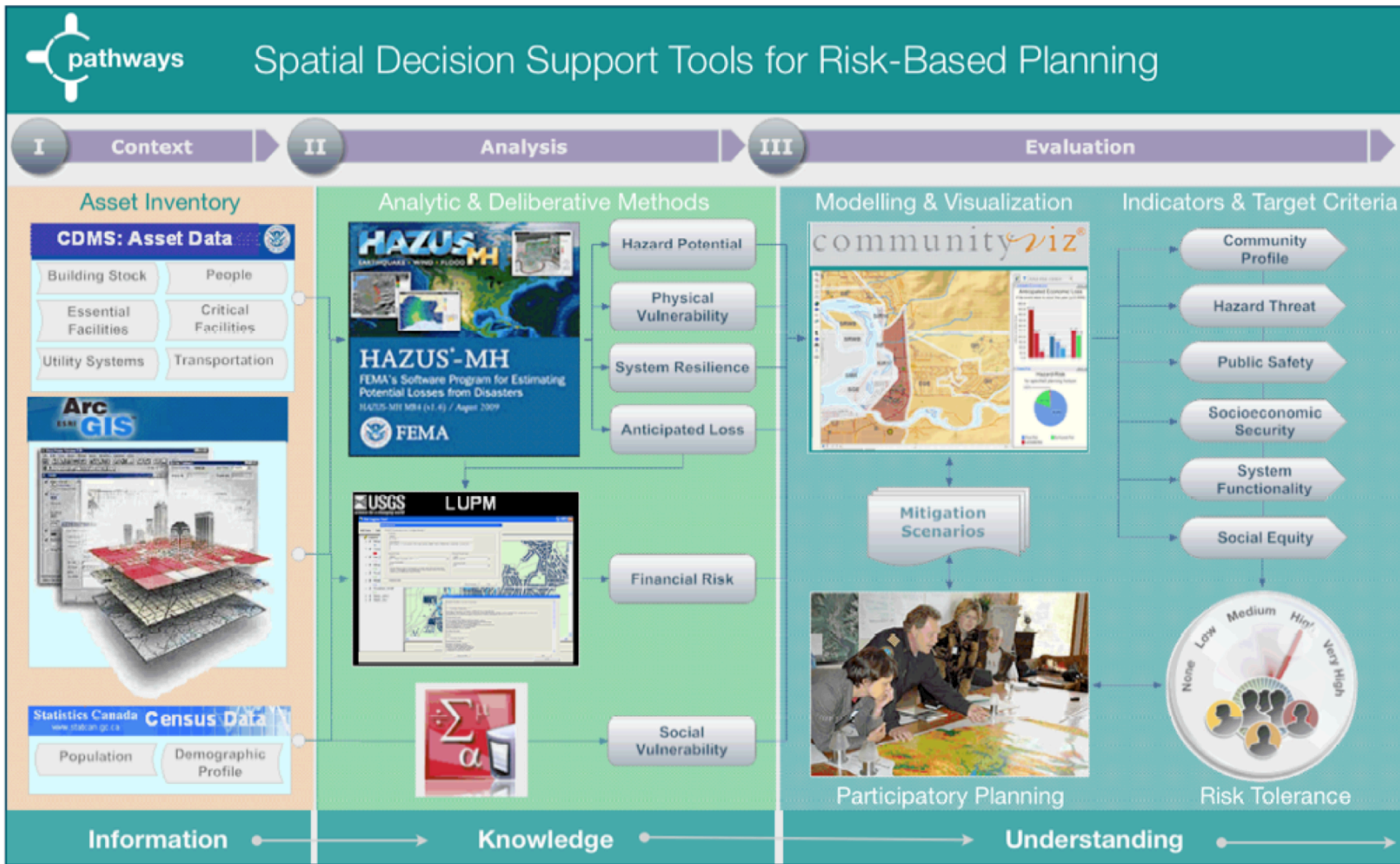
Figure 4-4: A schematic representation of the Pathways framework, implemented as a spatial decision-support system using available best practice methods and tools.
