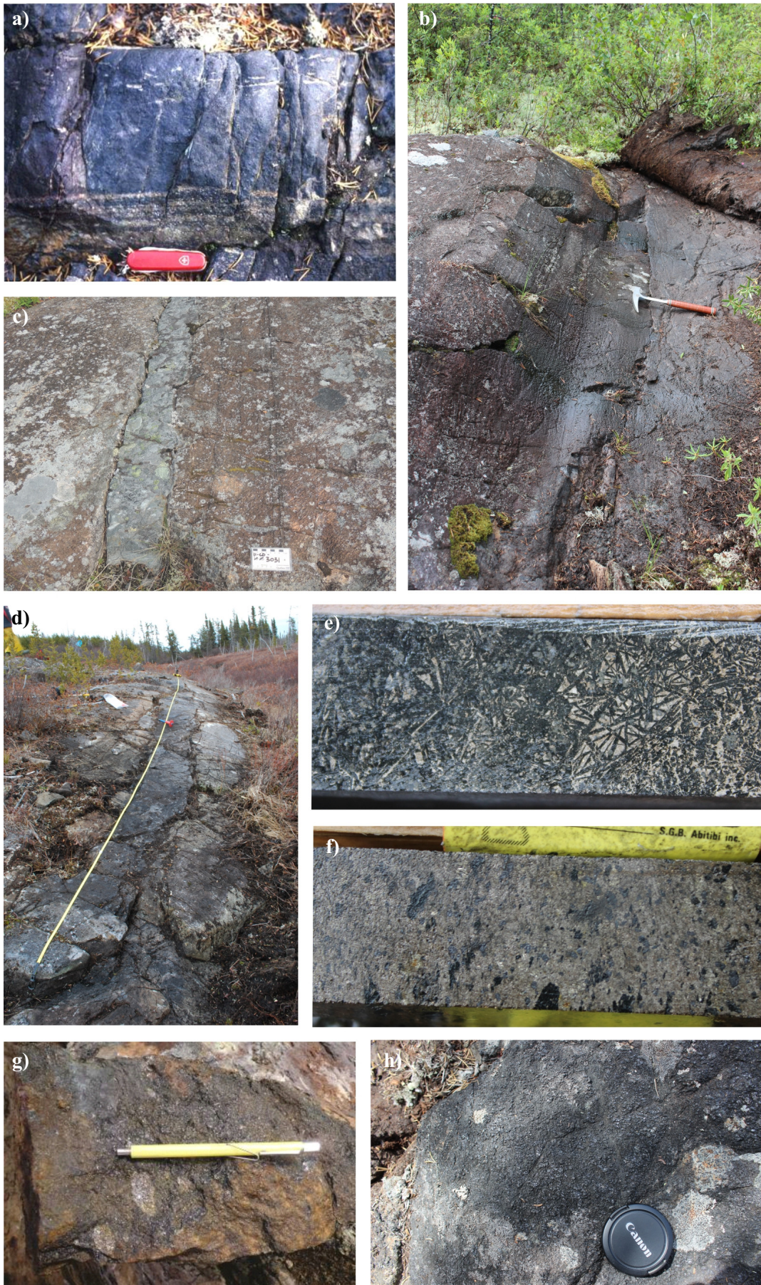
Figure 5. Typical examples of Cr-(PGE), Ni-Cu-(PGE), and Fe-Ti-(V) orthomagmatic mineralization observed in the La Grande Rivière and Eastmain domains. a) Chromitite and silicate chromitite seam from the Menarik Complex. Knife is 9 cm long. b) Massive and semi-massive chromitite seams from the Lac des Montagnes intrusions. Hammer is 30 cm. c) Thin massive chromite seam from the Lac Long intrusion. d) Massive chromite seam from the Lac Fed intrusion. Chisel is 24 cm long. e) Jack-straw-textured ore from the Nisk-1 deposit. Core is 4.5 cm in diameter. f) Massive to semi-massive sulphides from the Nisk-1 deposit. Core is 4.5 cm in diameter. g) Peridotite with disseminated sulphides containing cm-scale blebs of massive sulphides from the L occurrence in the Gayot area (courtesy of Mines Virginia). Magnetic pen is 12.5 cm long. h) Massive magnetite from the Baie Chapus Pyroxenite. Lens cap is 4 cm.
