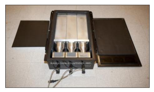
FIGURE 3 RSX-3 BOX WITH THREE 2" × 4" × 16" NAI(TL) CRYSTALS.
