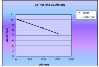
FIGURE 23 AMS RESULTS OF ALTITUDE SPIRAL OVER LAKE MOHAVE CALIBRATION RANGE. PLOTTED AS LOG OF NET GC.
