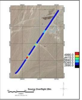
FIGURE 29 GROSS-COUNT RESULT FOR THE 30 M (~100FT) OVERFLIGHT.
