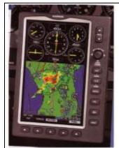
FIGURE 13 GARMIN 696 NAVIGATION UNIT AS USED BY NRCAN BY THE PILOT FOR SURVEY NAVIGATION.
