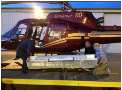
FIGURE 10 INSTALLATION OF THE NRCAN SYSTEM ON THE SUNDANCE AS350 HELICOPTER.
