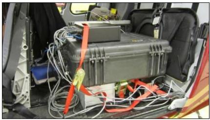
FIGURE 12 INTERALLY MOUNTED EQUIPMENT: ON THE BOTTOM TWO RSX-1 CRYSTALS AND RSN-4 NEUTRON DETECTOR; ABOVE THAT, THE BATTERY BOX AND POWER DISTRIBUTION SYSTEM WITH RS-705 CONSOLE ON TOP. THE POWER DISTRIBUTION SYSTEM AND CONTROLLING LAPTOP ARE BARELY VISIBLE BEHIND THE BATTERY BOX AND CONSOLE. EQUIPMENT WAS STRAPPED TO TIE DOWNS IN THE AIRCRAFT.
