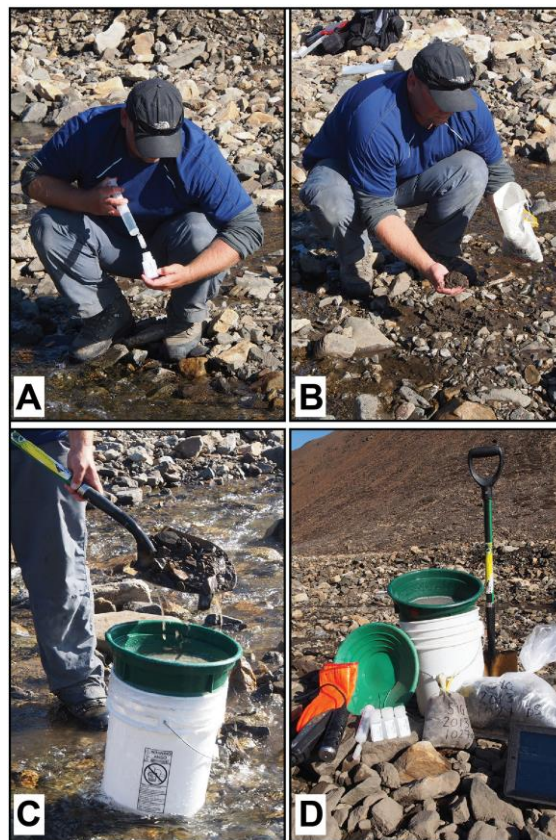
Figure 4. Sampling equipment and protocols: (A) Filtering water sample with 0.45 \mu\text{m} filter into 60 ml HDPE bottle. (B) Approximately 2 kg of wet silt and clay is collected from lower energy part of streams into a spun-bonded polyester cloth bag. (C) Approximately 12-15 kg bulk sediment for heavy minerals is collected by wet-sieving with a 2 mm mesh sieve in higher energy part of streams into large plastic bags. (D) Field equipment used and samples collected at a typical stream site.
