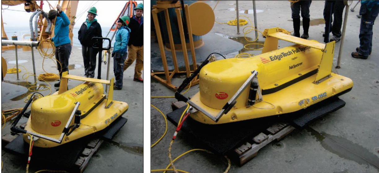
Figure 4. Chirp acoustic profiling system towed vehicle on the back deck of the icebreaker Healy.
