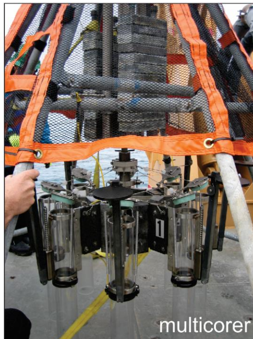
Figure 2. The Jumbo piston corer is (in the two left photographs) capable of collecting up to 25 m cores. The Multicorer, featured in the right hand photographs, can collect 8 short cores simultaneously.
