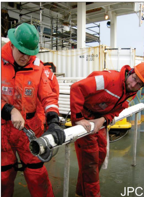
Figure 2. The Jumbo piston corer is (in the two left photographs) capable of collecting up to 25 m cores. The Multicorer, featured in the right hand photographs, can collect 8 short cores simultaneously.
