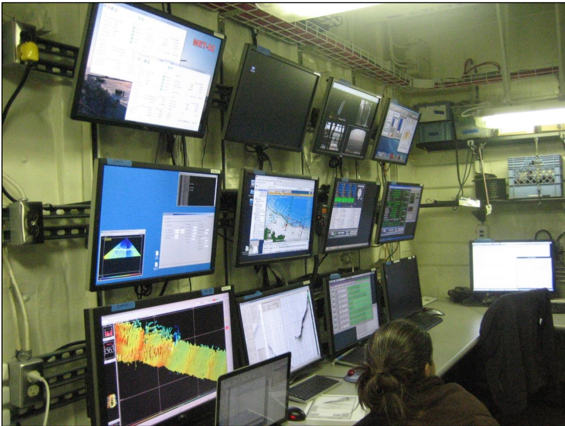
Figure 3. Multibeam, 3.5 profiler and positional data is collected in the geophysical lab.
