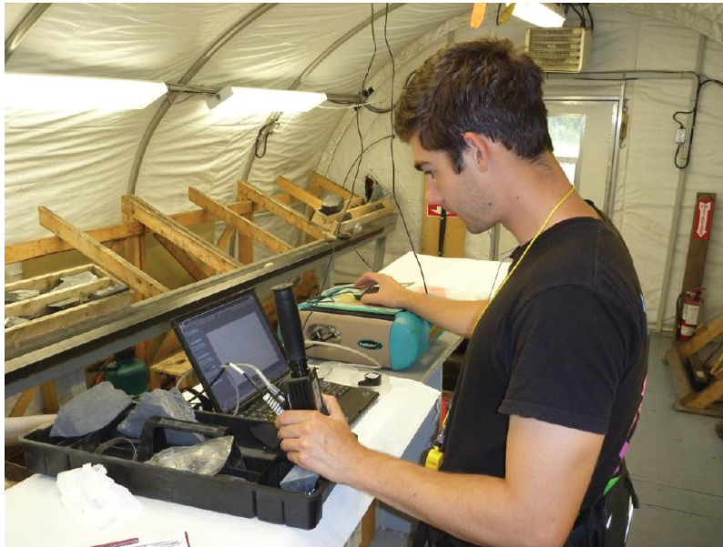
Figure 2. Collecting optical reflectance spectra from drill core samples with a field portable spectrometer in the Selwyn Chihong Mining Limited Don Camp core logging and sampling facility, Howard's Pass District, Selwyn Basin, Yukon.
