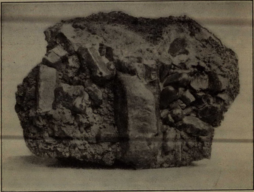
Group of apatite crystals, showing rounded, pitted and glazed faces. From township of North Burgess, Ont.
