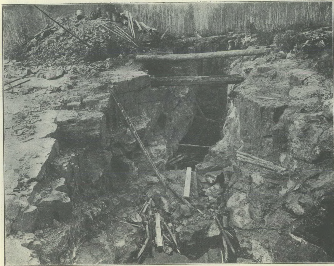
Open cut on apatite lead, McCrae mine, township of Templeton, Que. Ordinary method of working surface showings of phosphate and mica on vertical veins.
