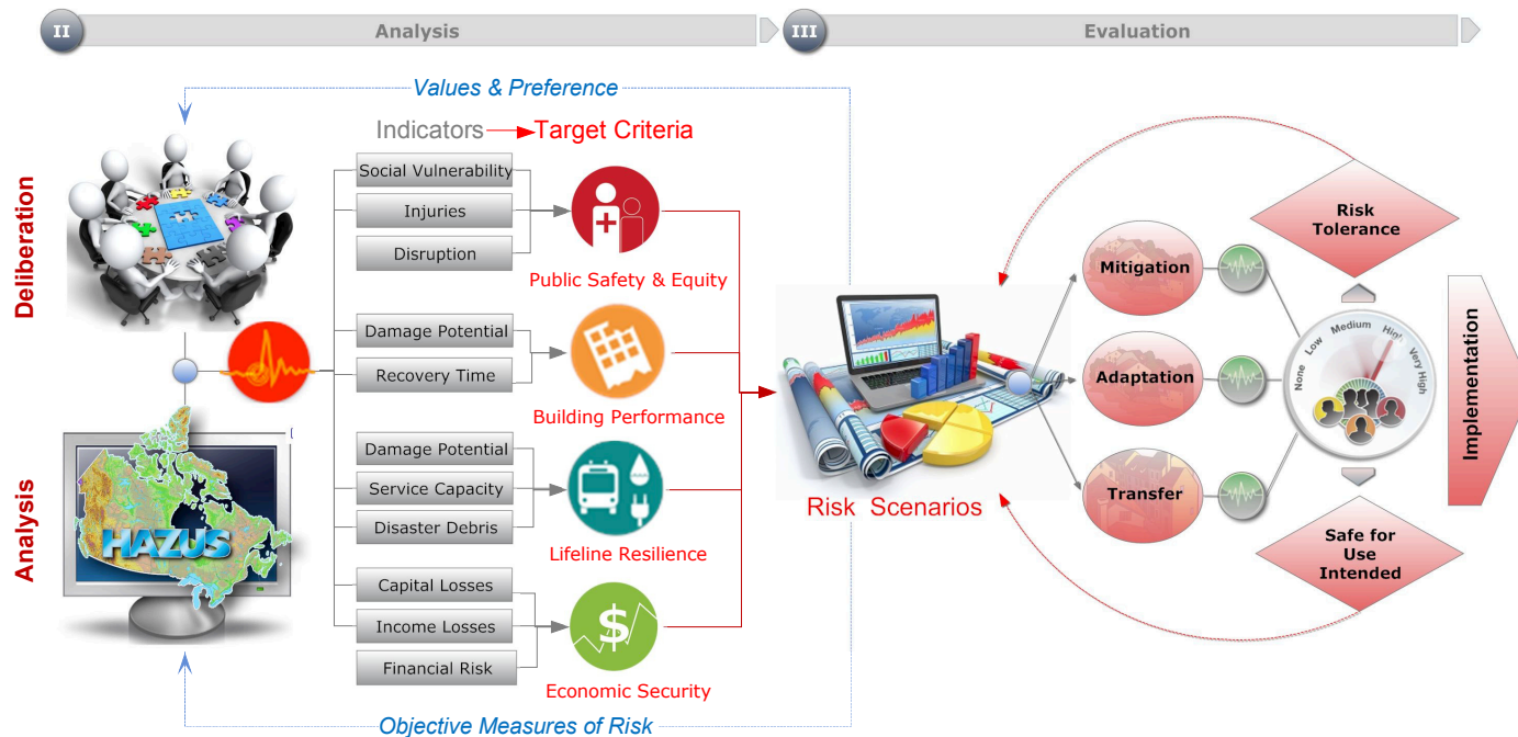
Figure 93: Analytic workflow for evaluating the strengths and weaknesses of risk scenarios using performance measures as a bridge between science, policy and decision-making
