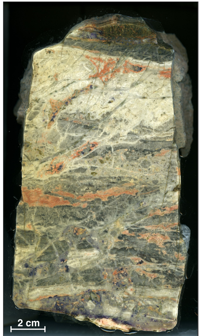
Figure 5. Adularia-rich epithermal agate sample, showing multiple episodes of brecciation and silica precipitation (sample 10PHA-01). Adularia occurs as orange (Fe-stained) stringers and sub-millimetre sized euhedral wedges (not visible) in early agate. Purple fluorite is present as late fracture filling. 2015-015.
