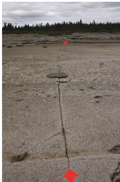
Figure 10: Example of a very continuous (>25 m) and linear fracture. Note that the fracture does not cut the overlying bed (dark patch in the central part of the photo). Near site MIN-11.
