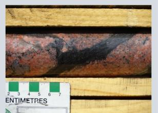
Fig. 4-D: Hydrothermal graphite vein cutting granite (WR-440)
