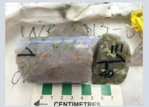
Fig. 4-B: Oriented sample of hydrothermal quartz (WR-440)
