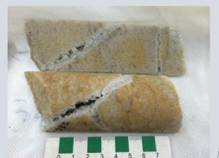
Fig. 4-F: Vuggy Quartz cutting sandstone (WR-250)
